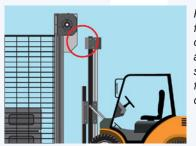
Rollback model – top roll behind the door for the need of a maximum compact cell, and highest possible safety with all moving parts inside the cell.
